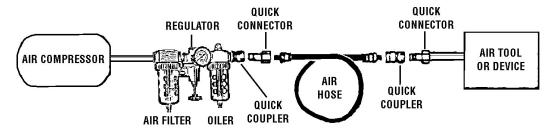
Connect the air tool, air hoses, filter, and oiler to the Compressor Air Outlet as illustrated below. Use pipe thread seal or Teflon tape on all threaded connections. The filter and oiler (not supplied) are recommended but not mandatory for operation.
